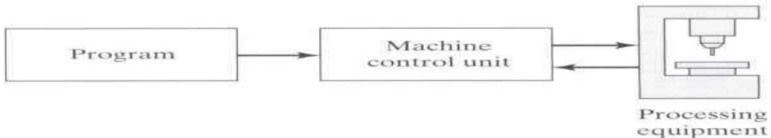
Figure 6.1 Basic components of an NC system.
